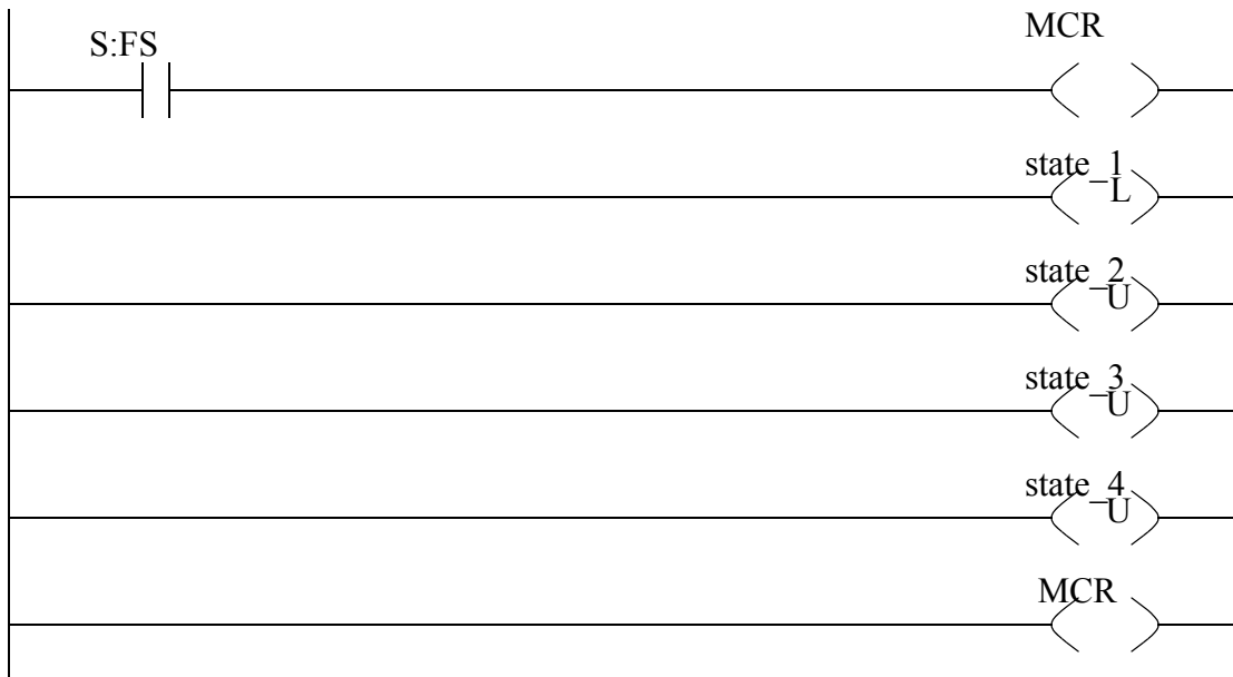
Figure 12.10 Ladder Logic to Initialize Traffic Light Controller
